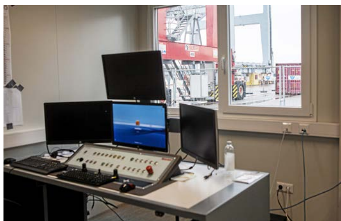
GOOD OVERVIEW: From the control desk, the operator will have a total of 12 different images from different cameras of the crane, thus a far better view than by sitting in the crane. cranes—to two or three in front of the remote control joysticks.
